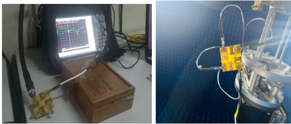
Figure 8. Fabricated prototype of 4-port multi-slot antenna a) front side b) backside
