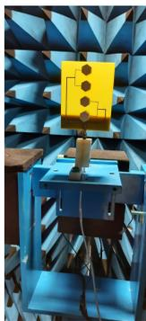
FIGURE 9: Anechoic chamber measurement setup.
