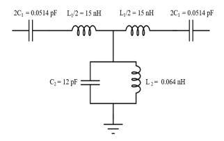
FIGURE. 6. EQUIVALENT CIRCUIT OF SYMMETRICAL RING RESONATOR BANDPASS FILTER.
