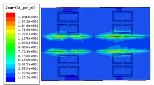
FIGURE. 11.A. THE CURRENT DISTRIBUTION OF SYMMETRICAL RING RESONATOR BANDPASS FILTER AT 5.7 GHZ FREQUENCY IN THE PASSBAND
