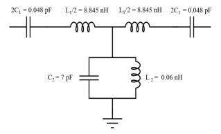
FIGURE.7. EQUIVALENT CIRCUIT OF MOORE FRACTAL APPLIED SYMMETRICAL RING RESONATOR BANDPASS FILTER.
