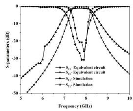
FIGURE. 10. S-PARAMETERS OF MOORE FRACTAL APPLIED SYMMETRICAL RING RESONATOR BANDPASS FILTER USING ELECTROMAGNETIC SIMULATION AND EQUIVALENT CIRCUIT SIMULATION
