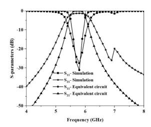
FIGURE.9. S-PARAMETERS OF SYMMETRICAL RING RESONATOR BANDPASS FILTER USING ELECTROMAGNETIC SIMULATION AND EQUIVALENT CIRCUIT SIMULATION.
