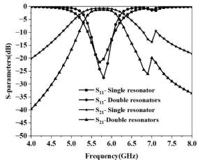
FIGURE.8. COMPARISON OF S-PARAMETERS OF BANDPASS FILTER WITHOUT FRACTAL USING SINGLE RESONATOR AND TWO RESONATORS.
