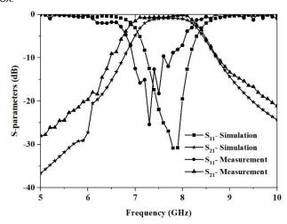
FIGURE.14. ELECTROMAGNETIC SIMULATION AND MEASUREMENT S-PARAMETERS FOR MOORE FRACTAL APPLIED BANDPASS FILTER.
