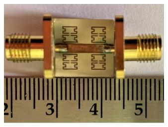
FIGURE. 13.A. TOP VIEW OF FABRICATED MOORE FRACTAL APPLIED SYMMETRICAL RING RESONATOR BANDPASS FILTER.
