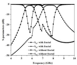
FIGURE. 12. S-PARAMETERS OF SYMMETRICAL RING RESONATOR BANDPASS FILTERS WITHOUT AND WITH MOORE FRACTAL.
