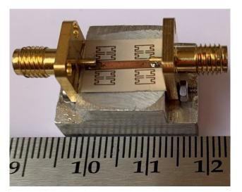
FIGURE. 13.C. TOP VIEW OF FABRICATED MOORE FRACTAL APPLIED SYMMETRICAL RING RESONATOR BANDPASS FILTER WITH MOUNTING BOX
