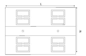
FIGURE.3. TOP VIEW OF PROPOSED SYMMETRICAL RING RESONATOR BANDPASS FILTER.
