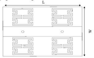
FIGURE. 5. TOP VIEW OF MOORE FRACTAL APPLIED SYMMETRICAL RING RESONATOR BANDPASS FILTER.
