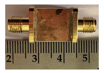
FIGURE. 13.B. BOTTOM VIEW OF FABRICATED MOORE FRACTAL APPLIED SYMMETRICAL RING RESONATOR BANDPASS FILTER.
