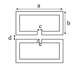
FIGURE 1. SYMMETRICAL RING RESONATOR UNIT CELL.
