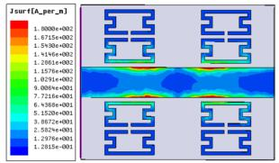
FIGURE. 11.B. THE CURRENT DISTRIBUTION OF MOORE FRACTAL APPLIED SYMMETRICAL RING RESONATOR BANDPASS FILTER AT 7.8 GHZ FREQUENCY IN THE PASSBAND.
