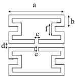
FIGURE. 4. THE UNIT CELL OF THE MOORE FRACTAL APPLIED SYMMETRICAL RING RESONATOR.
