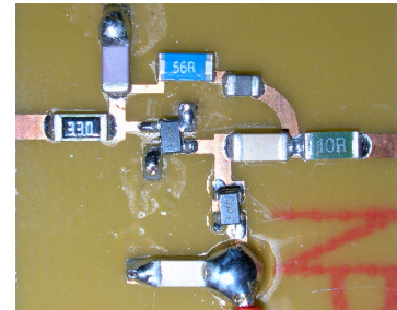
Figure 17: Photograph of the RCNGD-circuit implemented.
