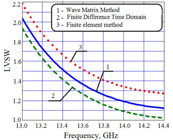
FIGURE 4. LVSW versus frequency for horizontal polarization
