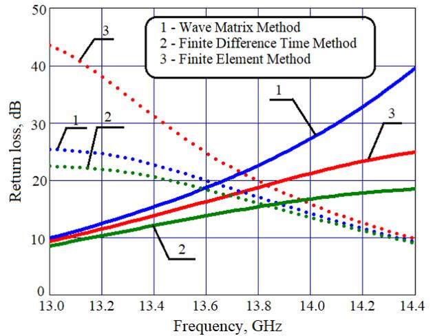
FIGURE 8. Frequency dependence the return loss for a polarizing device
