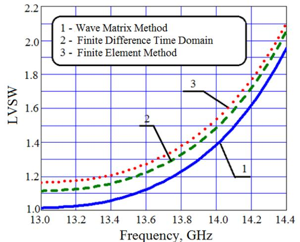
FIGURE 5. LVSW versus frequency for vertical polarization
