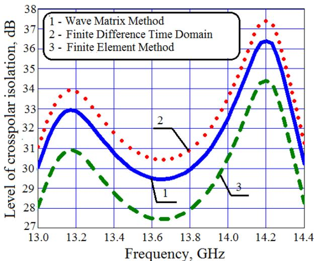
FIGURE 7. Frequency dependence the LCI for a polarizing device
