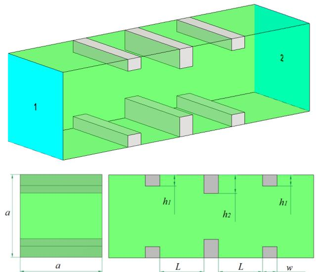
FIGURE 1. Inner structure of the square guide polarizer with 3 diaphragms
