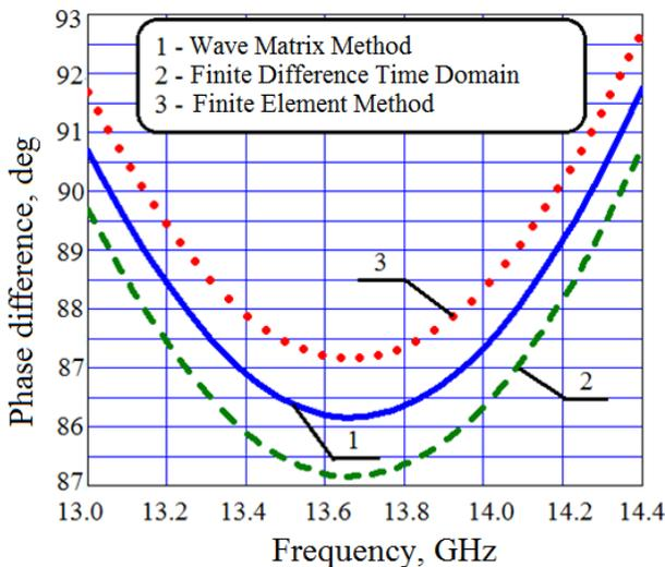
FIGURE 3. Phase differential versus frequency
