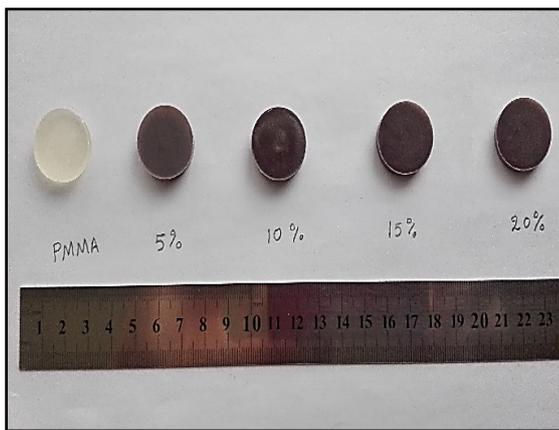
Figure 3: Dielectric test specimens at a different weight fraction
