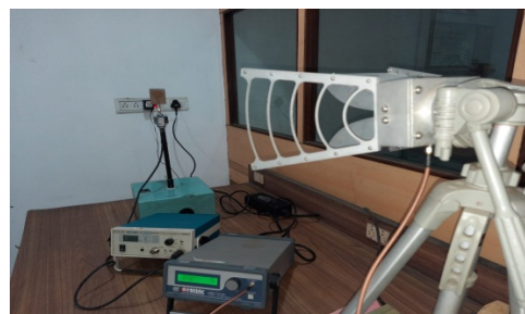
FIGURE 8. Experimental setup for the measurement of the radiation pattern
