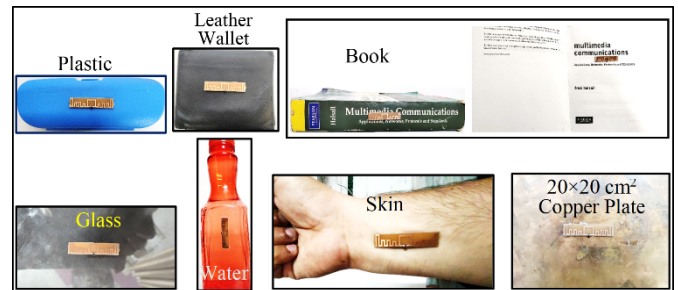
FIGURE 19. The proposed tag placed on/in different materials.
