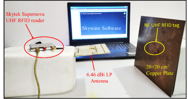
FIGURE 18. Setup for measuring the reading range and reading rate of the proposed tag.
